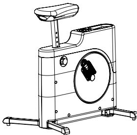
Take the seat up by turning the wrench counter clockwise. Once the seat is in the desired position, tighten the wrench clockwise.
